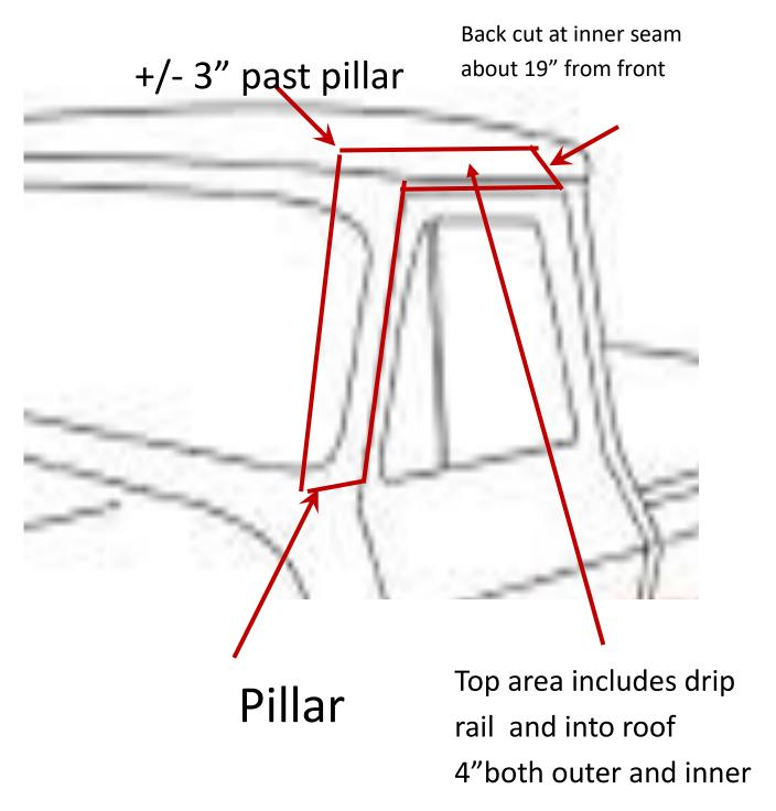
You can separate the pillar from roof section for ease in packing and shipping
