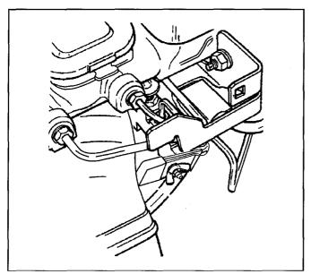
Figure 9—Depressing Combination Valve
