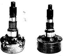
The above sectioned drawing shows the DNE<sup>2</sup> 2 by 4 conversion shaft in its installed position. To the left, the two versions of stock components that it replaces.
