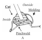
Cut inner lip off of weatherstrip above the pinchweld (diagram A). Use a flat teflon knife or spatula to release the rubber from the glass and the body. Carefully push the glass from the inside upper corners and center, applying even pressure. Do not over push. If you do not feel the glass starting to give, then check the weatherstrip, both inner and outer, to make sure that it has released from the body and is clear of the pinchweld. It should remove easily.
