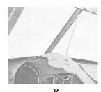
Lubricate the 1/4" glass groove with glass lubricant or very soapy water to allow the glass to center itself while installing. Place new rubber on glass making sure that it is placed correctly and fits well. Any problems with fit will show up at this point. Rubber should fit glass without being too loose or too tight. Improper size will pucker or fold in corners. Place chrome strips in top and bottom slots of rubber first. Next, position sides and lock-in corners. Place 1/8" cotton cord
